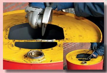
Due to the fact that the washer does not fit through the holes made, grind or saw the intermediate piece between the 2 holes.
