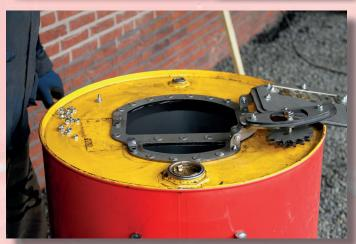
Now attach the front plate with door onto the barrel. Fix it by placing the back place inside the barrel using the nuts and bolts.
