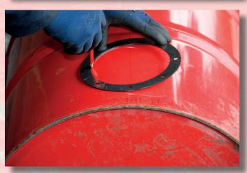
Place the barrel on its front legs. Mark the hole and mounting holes of the flue on the back of the barrel.
