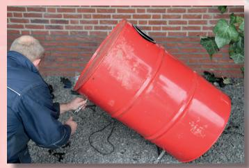
Place the second pair of legs through the hole of the flue pipe at the back end of the barrel.
