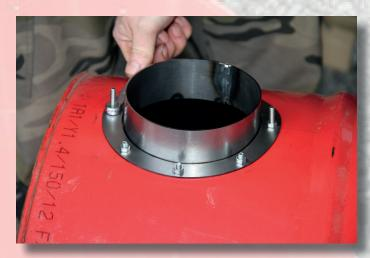
Place the inner plate and the ring in the hole for the flue pipe and fix them with the long bolts. This will pull the inner plate, the barrel and top ring together.
