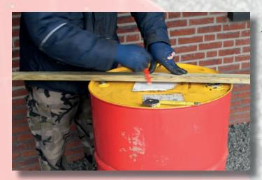
Decide what the center of the barrel is. This allows you to determine the correct position of the door, legs and flue pipe.
