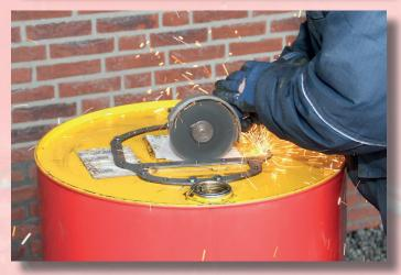
Mark the inside of the washer and remove those marked parts with a grinder...
